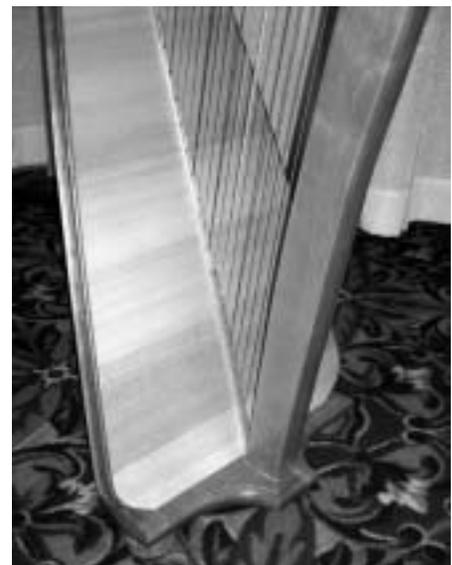
Note how the extend soundboard returns to meet the body at the bottom of the instrument. This close-up shows the inlay banding and router grooves that Lee added to enhance the appearance of the side molding.
