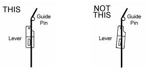
When the lever is placed correctly, go ahead and drill the pilot hole (7/64") bit) for the mounting screw in the middle of the slot. Yes, you can do this without removing the lever or pushing the string to one side!
