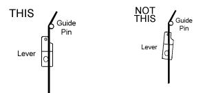
When the lever is placed correctly, go ahead and drill the pilot hole (7/64" bit) for the mounting screw in the middle of the hole. Yes, you can do this without removing the lever or pushing the string to one side!
