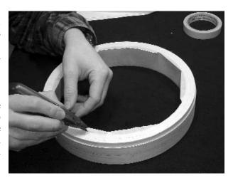
\_\_\_\_\_\_3. Using your square and a pencil. Draw a line connecting the centers of the two coordinator rod holes already drilled into the RIM.
