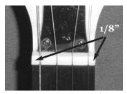
\_\_\_\_\_28. Attach strings number 1 and 5 first. Then you can install the bridge. The bridge will be located roughly 26 1/2" from the front of the nut. (You will fine tune this later).
