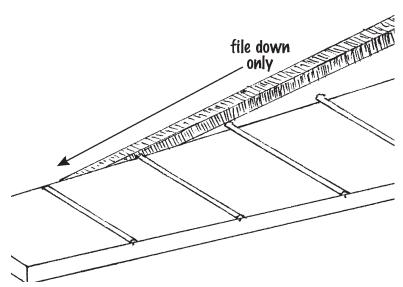
\_\_\_\_\_10. Once the frets are installed you need to file the ends flush with the fretboard. Always work the file in a downward motion, as shown, so you don't inadvertantly lift the end of a fret.
