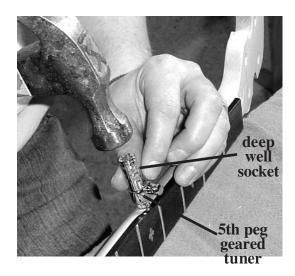
\_\_\_\_\_21. Note that there are two left-hand geared tuners and two right-hand ones. Install these tuners as shown in the picture. Use the threaded sleeve to secure the tuners on the front side. Then drill 1/16" pilot holes in the back side for the tiny screws. Put some masking tape on the drill bit as a depth guide so you don't accidentally drill all the way through the peghead.
