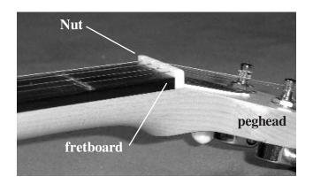
\_\_\_\_\_22. Test fit the nut to see that it will seat completely against the peghead and the fretboard. The nut will likely be taller than needed. It only needs to be 1/16"
