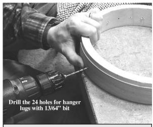
**HINT** - If you don't have brad-point drill bits, drill a pilot hole with a 1/8" bit first, then come back and re-drill with 13/64" bit.
