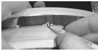
\_\_\_\_\_5. Directly opposite the two predrilled coordinator rod holes, you'll see that two of your pencil marks are spaced farther apart than all of the other marks. This wider space will accommodate the tail-piece and the other end of the coordinator rods.
