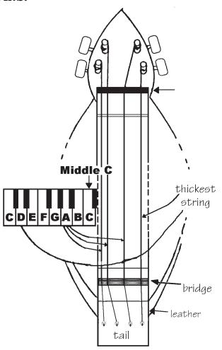
Pound the tail pins into place, leaving about 1/8" standing above the surface of the wood.
