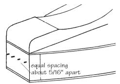
small holes in the TAILPIECE, as shown, for the TAIL PINS.
