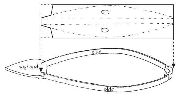
13. Prepare for gluing the SOUNDBOARD to the dulcimer body, taking care to orient it correctly:
