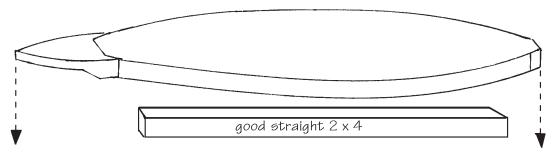
21. In order to glue the FRETBOARD in place, you will need to support the inside of the SOUNDBOARD with scraps of wood or something (an old 2 X 4 would do
