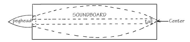
NOTE: The SOUNDBOARD should extend over the PEGHEAD far enough to cover the slots, as shown.
