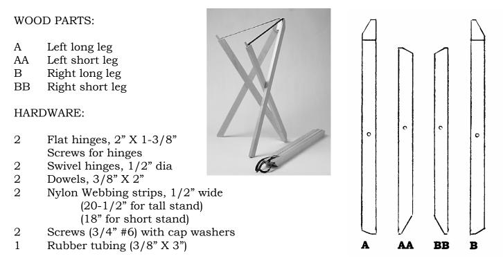
**CAUTION**: The wood parts of this kit are so similar that it is difficult to identify right from left. **Carefully lay out the pieces according to the diagram and then mark each piece as shown.** *If* you assemble these pieces incorrectly your stand will not work.
