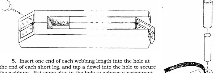
the end of each short leg, and tap a dowel into the hole to secure the webbing. Put some glue in the hole to achieve a permanent fit. Then cut the rubber tubing in half and slip one piece over each dowel for padding to protect your instrument.
