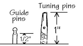
\_\_\_\_31. Pound the TUNING PINS into the upper row of the holes into the neck, using the <u>five with the</u> <u>enlarged holes in the front of the harp where the</u> <u>thickest (.060" diameter) strings will be.</u>
