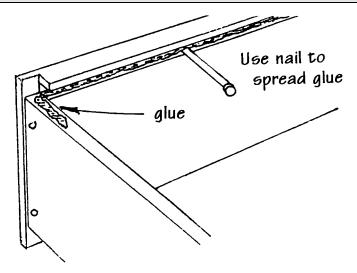
Lift the bottom lip of the SOUNDBOARD and squirt some glue under that as well. Then use several of the small nails provided to secure the SOUNDBOARD to the BASE. It's a good idea to add a couple of extra nails near the notch, as shown, because there is a lot of tension and stress at this point. (Don't worry, the nails will be covered over later).
