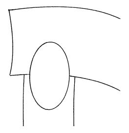
When the first OVERLAY piece has dried for at least 30 minutes, you may remove the clamps and put the other one in position on the other side so it mirrors the first. Clamp it in place until dry.
