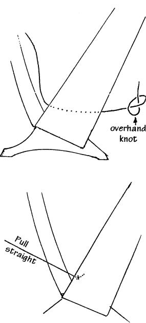
Turn the PIN clockwise with the tuning wrench as you take up the slack with the other
