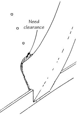
Look carefully at the back end of the NECK as well. We like the NECK to fit the top of the soundbox nicely too. Again, you may use a disk sander to adjust the back of the NECK or the top of the soundchamber, if necessary.
