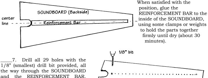
and the REINFORCEMENT BAR. These holes are drilled straight down at each punch-mark, not at an angle. NOTE: If you ordered the Optional
