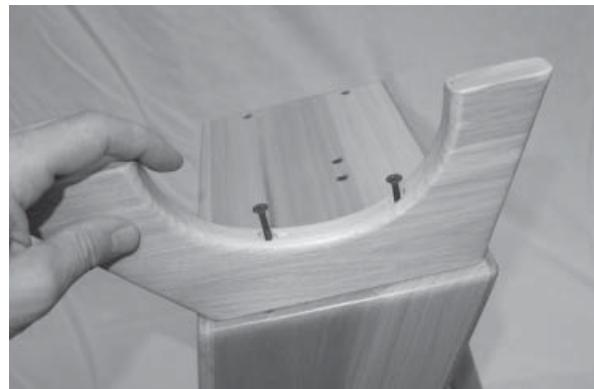
\_\_\_\_\_32. Using the punch marks as a guide - drill pilot holes into the **BASE** using the 1/8" drill bit.
