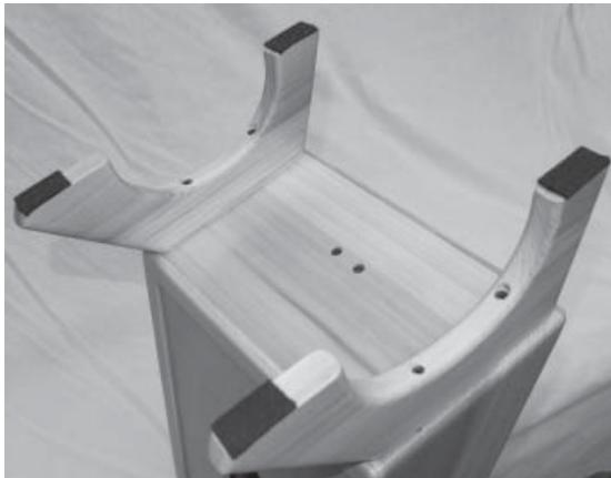
\_\_\_\_\_33. Cut the adhesive backed felt and stick to the bottom of the feet as shown to prevent scratching the floor, and to reduce the noise when you slide your harp into playing position. The pads should be positioned at each end for greatest stability.
