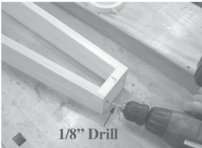
4. When the pilot holes are all drilled, remove the tape and put glue in the joints before installing 1-5/8" screws to draw the parts together permanently. Glue and screw both the **TOP** (2 screws) and **BASE** (4 screws) pieces to the sides. The screws should pull the parts together fully so that some glue squeezes out of the joints.
