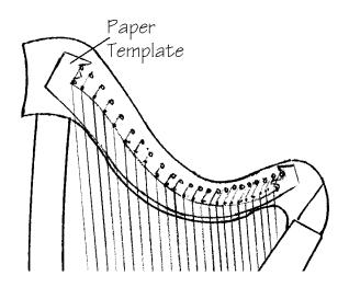
If you cannot obtain a template for lever placement on your harp, or you already have some levers mounted on the neck so you cannot use the template, make sure the instrument is perfectly tuned and stable before installing levers. You will rely on the pitch of the strings to determine the exact location of the levers. Read through to special instructions on next page.
