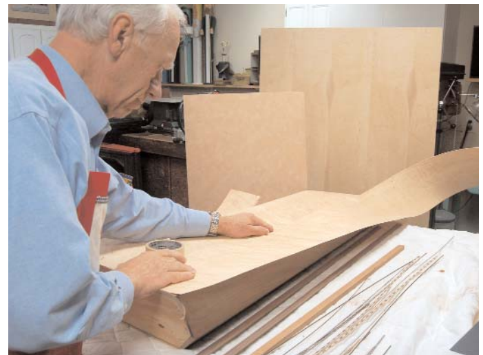
Chuck Story glues book-matched veneer sheets of curly maple together down the centerline of the soundboard.
