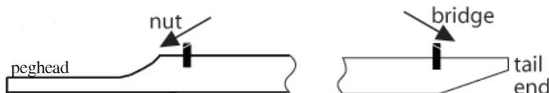
**19.** Now you can begin stringing. Notice that we have color-coded the ball end of each string. Install one string at a time by sliding the wire through the slot in the tail end of the string board.
