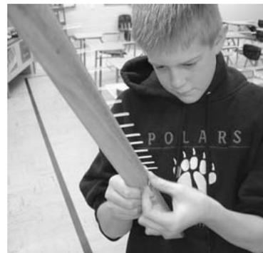
**16.** GENTLY sand the frets flush with the edge of the stick. This is best done with a flat sanding block or stick. Be sure to work the sandpaper downward only, so you don't lift the frets off.
