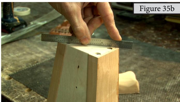
39) Orient the arched cap block on top of the harp and check for best fit. Use two 2-1/2" wood screws and a hammer to make punch marks into the top block for locating your pilot holes. Notice that the back of the block is taller than the front. (Figure 36)
