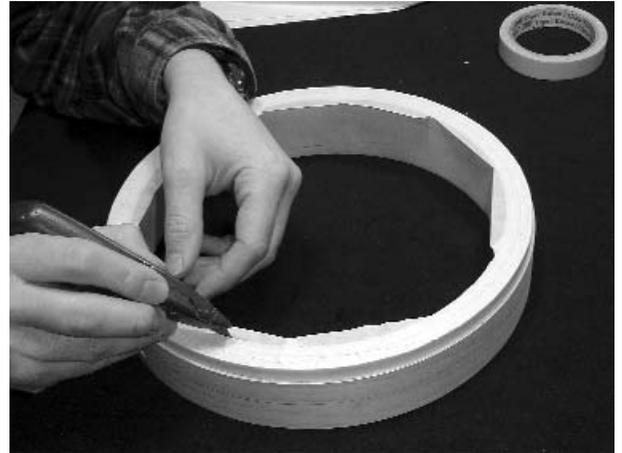
\_\_\_\_\_2. Check to see if your banjo RIM has a pencil line drawn around the outside. If it does, you can skip to step three. If not, you will need to add one. Mark a line all the way around the circumference of the RIM that is one inch from the bottom. (The top of the RIM is the part that you have taped off.)
