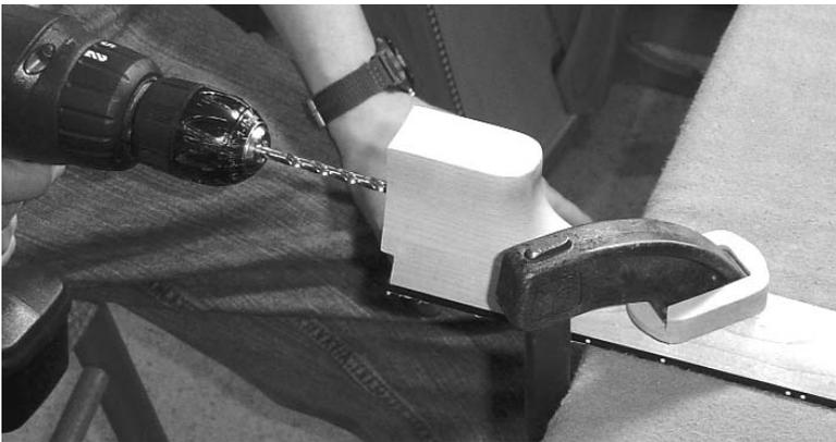
\_\_\_\_\_17. Remove the NECK from the body and clamp it to a sturdy table with your new clamp. Drill a  $\frac{13}{64}$ " pilot hole for the lag bolt. Drill straight to a depth of at least one inch, to match the wood threads of the hanger bolts.
