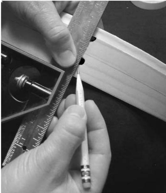
\_\_\_\_\_3. Using your square and a pencil. Draw a line connecting the centers of the two coordinator rod holes already drilled into the RIM.
