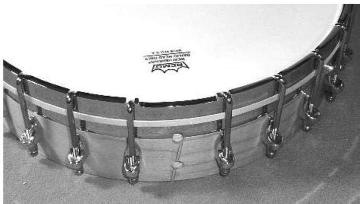
15. Assemble the pot as follows: Place the TONE RING on the RIM lining up the notches with the holes at each end. Then place the Skin Head over the TONE RING (we like to orient the printed logo toward the neck).
