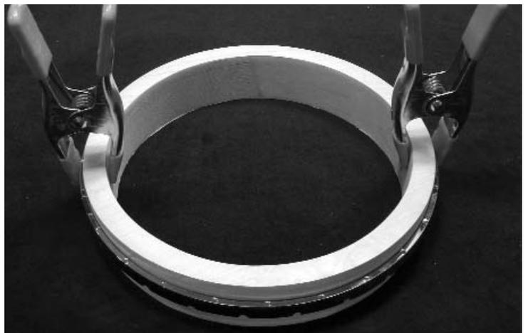
Double check that the TENSION HOOP is clamped securely and that the notches are lined up on the line around the RIM. Now you can carefully mark the center of each notch where it intersects the circumference line.
