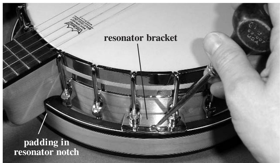
\_\_\_\_\_38. Now set the banjo assembly onto the resonator and use an awl to mark the location for the threaded inserts. Use a drill bit that is the exact size of the outside diameter of the insert, not counting the little burrs. Drill the holes slightly deeper than the insert is tall. Use a hammer to gently tap a threaded insert into each hole until fully seated. Attach the resonator to the pot assembly using the 4 knurled screws provided.
