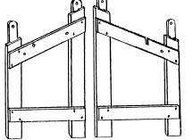
protrude above the tops of the legs. Insert the longer **BACK** SLIDES into the BACK LEGS in the same way. (There is no right or left for those sliding parts.)
