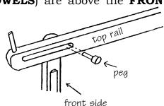
or left. Place the **WOODEN PEGS** into the holes and slots of the TOP RAILS, as shown.
