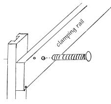
**\_\_\_\_13.** Insert the four **CARRIAGE BOLTS** into the **CLAMPING RAILS**, and tap the heads of the bolts firmly against the inside surface of the **CLAMPING RAILS**.
