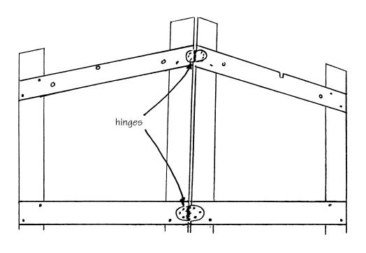
\_\_\_\_\_11. Before sliding the movable parts back into the stand, install the spring-loaded **HINGES** to the **BACK LEGS**. Actually, the hinges fasten to the **RAILS** instead of the legs, as shown.
