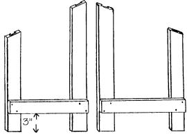
C) Position the BOTTOM RAILS 3" from the square bottoms of the **FRONT** & BACK LEGS. Do not fasten in place yet -just lay them in position for now.
