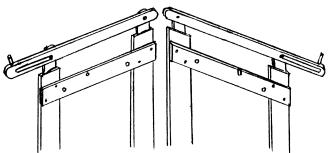
Position the two TOP RAILS on the 5. **SLIDING RAILS** so that the slotted ends (where you glued the **DOWELS**) are above the **FRONT**
