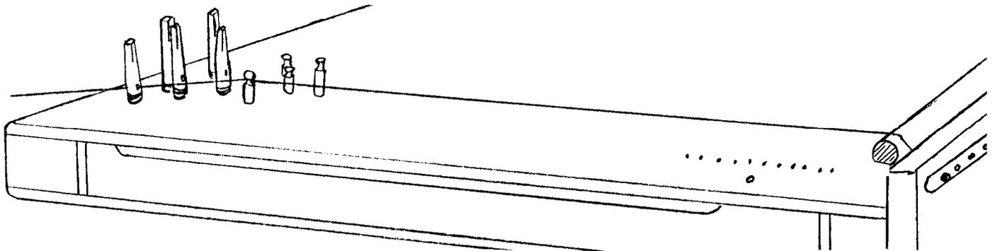
Pull the wire across to the last TUNING PIN near the point of the instrument, and push the end through the small hole in the pin.
