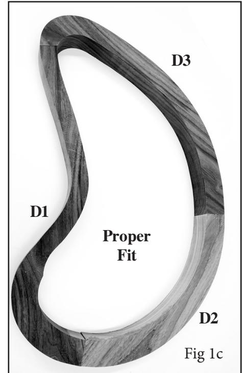
Then set the back panel aside and place the three frame pieces together. If the joints do not match correctly (Fig 1b), flip part D2 end-for-end and try again. You want the frame to look like Fig 1c.
