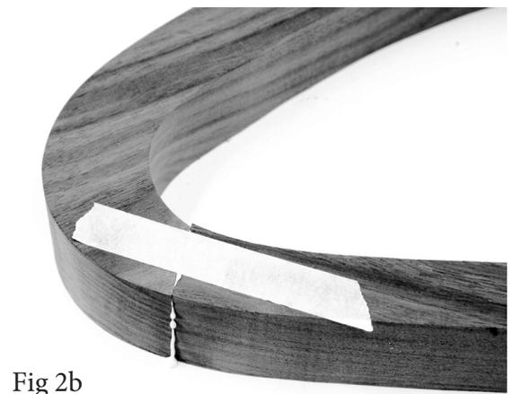
Put glue on both ends of part D2 and tape those two joints in the same way, as shown below. Add tape to the inside and outside surfaces of each glue joint, but don't bother turning the frame over to tape the other side -- that's not necessary.
