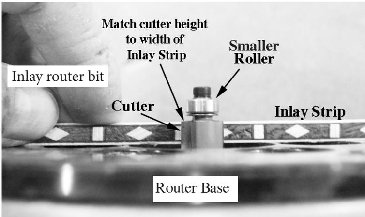
When ready, hold the router base flat on the front of the box as you rout the ledge around the circumference. Go around 2-3 times, just to make sure you have cut to the full depth all the way around the instrument.
