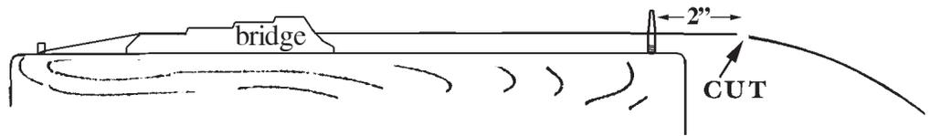
**B.** Pull the end of wire back and insert it into the tuning pin so it just barely shows through the other side of the pin, as shown at right.
