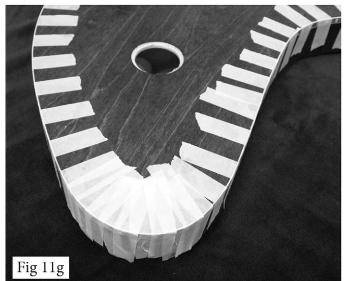
12. Now is the time to do some rounding of the edges on the instrument. If you installed inlay banding around the top, you don't want to round that edge, but you can put a generous round-over on the back edge (unless you went around the back with inlay too). If you skipped the inlay banding part of the project, you'll want to round over both the front and the back edges of the box.
