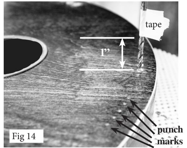
Wrap masking tape around the drill, 1" from the tip, as shown at right. This will guide your drill to the correct depth for each hole. You may use either a drill press or a hand drill (electric or battery) to drill these holes. They should be as straight (vertical) as you can make them at each punch-mark near the edge of the instrument.
