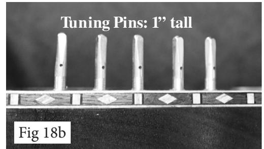
If you don't have a drill press, you can actually screw the pins into place using the Allen wrench and Tuning Key provided, though that is a bit tedious. It would be faster to use a hammer, placing a scrap of wood beside the pin as you pound, to help prevent damaging the finish in case the hammer slips. A smart thing would be to make your wood scrap the desired height for the pins, so you pound or screw or press until the top of the pin matches the top of the scrapwood.
