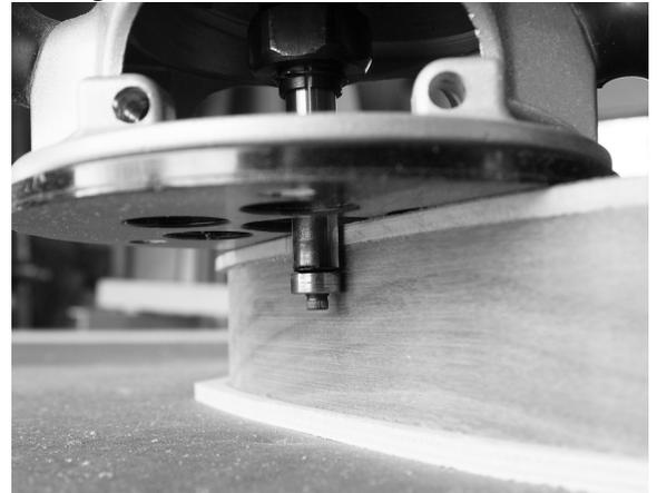
8. Notice that the flush-trim bit probably left a few bumps of glue residue and jumped a little at the glue joints in the frame, so you need to do some sanding to smooth the edges of the box more completely. If you don't have a belt sander, and need to work by hand, make a flat sanding block with coarse (80-100 grit) sandpaper for this job of cleaning up the edges and smoothing the glue joints.
