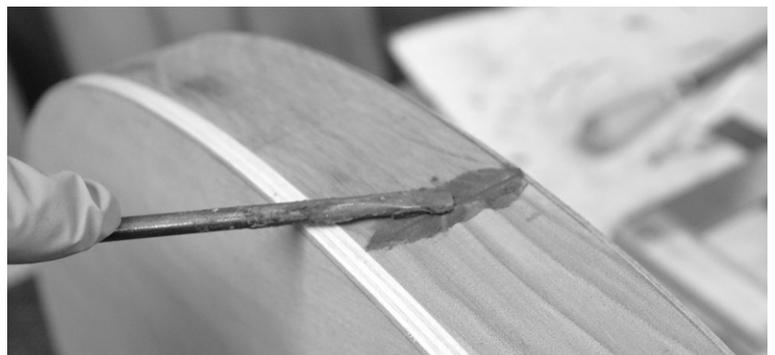
Now you need to decide if you wish to go gung-ho by customizing your instrument with inlay banding or not. It takes a smaller roller for the flush-trim router bit to cut a ledge around the circumference of the box for inlay banding. This is purely optional, and it adds a number of hours and some careful detail work to the project.
