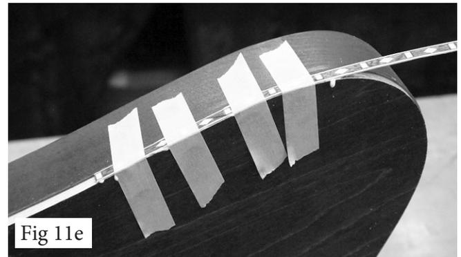
When you come to the sharpest curve on the instrument, handle the inlay gently so it doesn't break when wrapping around this tight curve. Use a wet rag to dampen the next 6 inches of inlay strip (both sides) to make it more pliable. The water will soften the wood and make it flex more easily.
