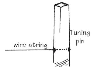
**C.** Use the tuning key to turn the pin clockwise about 1/2 turn, leaving the string loose enough so it does not pull out of the little hole.
