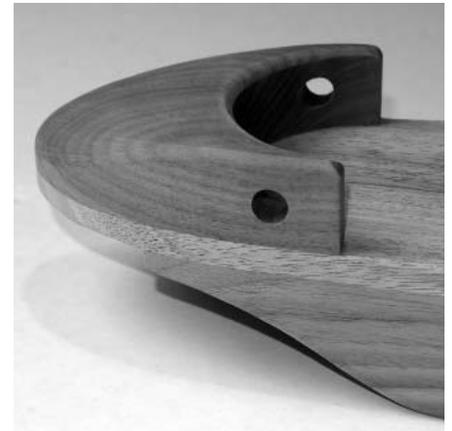
Finally, go over the entire instrument by hand with some 180 grit sandpaper until you have a nice smooth surface and there are no visible machine marks or glue spots.
