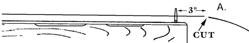
**B.** Pull the end of wire back and insert it into the tuning pin so it just barely shows through the other side of the pin, as shown. This will prevent the sharp end from poking your skin or snagging your clothes.
