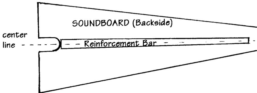
When satisfied with the position, glue the **REINFORCEMENT BAR** to the inside of the **SOUNDBOARD**, using some clamps or weights to hold the parts together firmly until dry (about 30 minutes).
