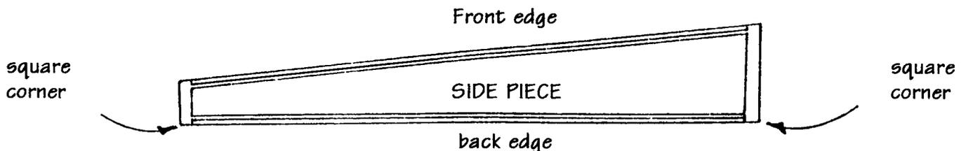
⇒ The front edge of each SIDE is cut at a slight angle, whereas the back edge is square relative to each end.
