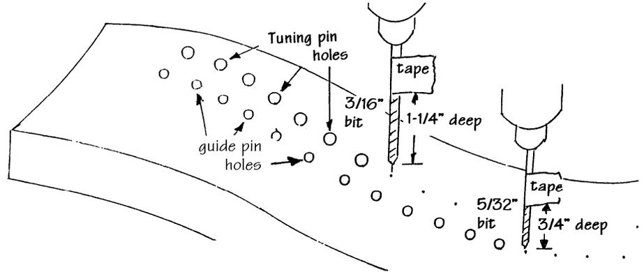
HINT: Wrap masking tape around your drill bit leaving 1 1/4" exposed.
