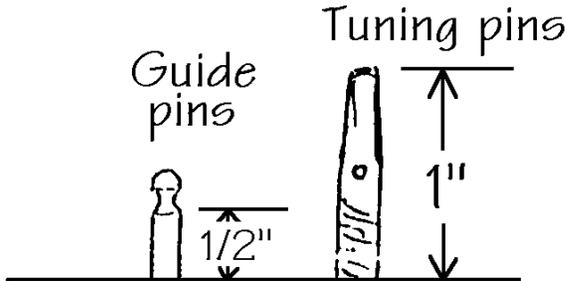
\_\_\_\_31. Pound the TUNING PINS into the upper row of the holes into the neck, using the five with the enlarged holes in the front of the harp where the thickest (.060" diameter) strings will be.
