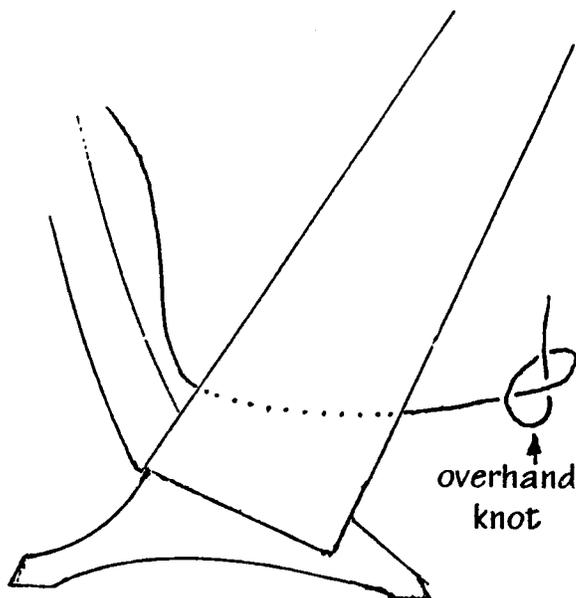
NOTE: PULL STRAIGHT THROUGH THE HOLE, NOT AT AN ANGLE, SO AS TO AVOID SCRATCHING THE NYLON AGAINST THE BRASS EYELET.
