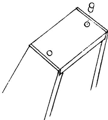
\_\_\_4. Glue two CHERRY WOOD PLUGS into the TOP, covering the screws, just for looks. Sand these plugs flush with the surface of the TOP when they are dry.
