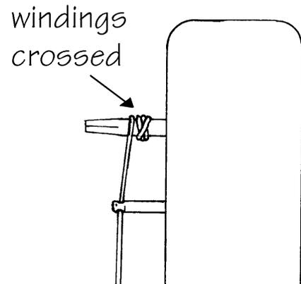
**IMPORTANT:** It is necessary to also anchor the tops of these .040" strings (and all the lighter ones) securely to the tuning pins, as follows:
