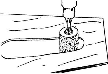
HINT: A drum sanding attachment to your drill (2" diameter, #80-grit sandpaper) is a great little tool for eliminating the rough spots and rounding things out.
