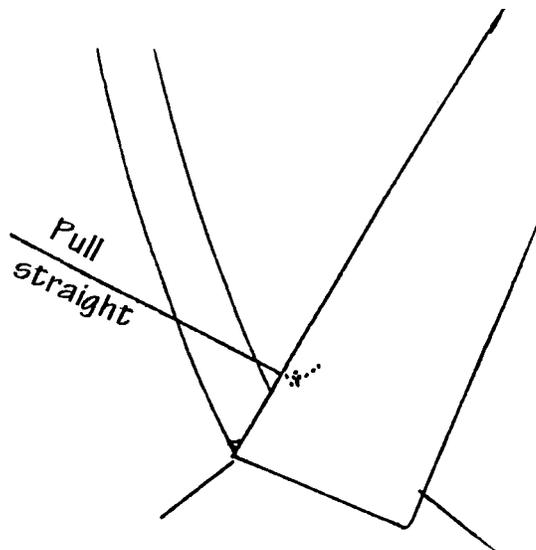
Turn the PIN clockwise with the tuning wrench as you take up the slack with the other hand, guiding the string as it winds around the pin. As the string begins to tighten, place it in the groove of the GUIDE PIN.
