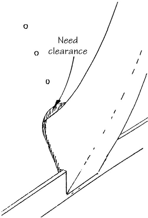
Look carefully at the back end of the NECK as well. We like the NECK to fit the top of the soundbox nicely too. Again, you may use a disk sander to adjust the back of the NECK or the top of the soundchamber, if necessary.
