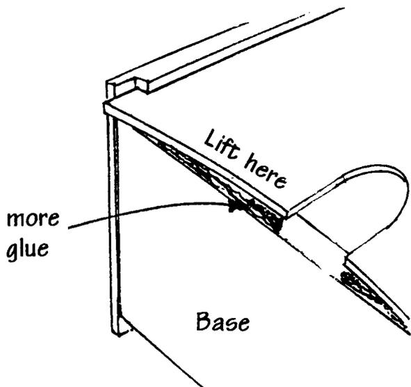
Lift the bottom lip of the **SOUNDBOARD** and squirt some glue under that as well. Then use several of the small nails provided to secure the **SOUNDBOARD** to the **BASE**. It's a good idea to add a couple of extra nails near the notch, as shown, because there is a lot of tension and stress at this point. (Don't worry, the nails will be covered over later).
