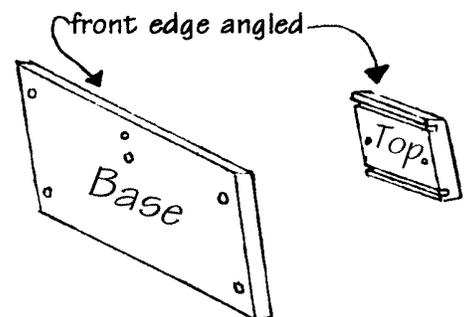
\_\_\_2. When satisfied with the fit, use a 7/64" drill bit to bore pilot holes through the TOP piece into the SIDES so that the screws will draw the parts together firmly. Assemble the TOP to the SIDES with glue and screws (1-5/8").
