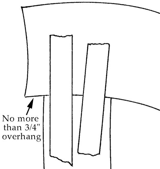
\_\_\_22. With the NECK and PILLAR resting in position on the harp, glue the NECK to the PILLAR, using masking tape to hold the parts still until dry. No, this is not a very sturdy joint yet, but you will be adding OVERLAYS to the outside of this joint next.
