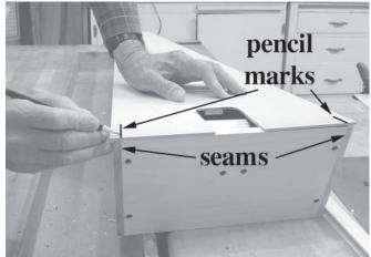
\_\_\_\_\_13. Then use a straight-edge (or straight piece of wood trim from your kit) as a guide to draw lines connecting these marks along both sides of the SOUND-BOARD. These will be the lines that guide your nailing. We don't want any nails to poke out of the wood!
