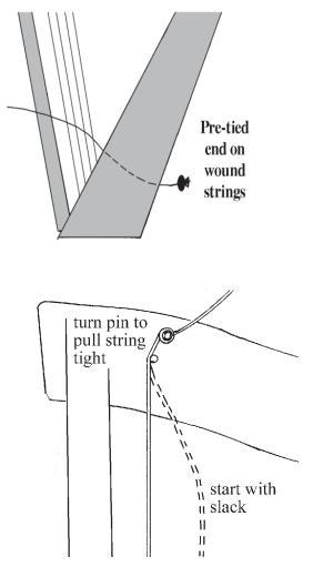
When you come to the first plain nylon string (.050" diameter), push it through from the front of the harp and pull the end partway out the back of the harp, so you can thread a plastic bead onto the string and tie a simple overhand knot, as shown.
