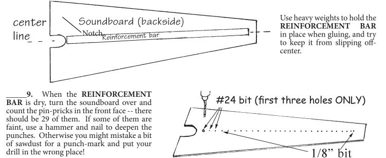
Use the #24 drill bit to drill just the first 3 holes (nearest the notch) through the **SOUNDBOARD**. This is the larger bit in your kit. Drill all the way through the **REINFORCEMENT BAR** too. Then switch to the smaller 1/8" bit to drill the remaining 26 holes.
