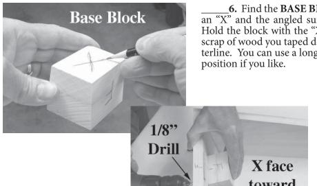
**6.** Find the **BASE BLOCK** and mark the smallest surface with an "X" and the angled surface with the letter "**F**", as shown here. Hold the block with the "X" against the **BASE**, next to (under) the scrap of wood you taped down as a guide, and center it on your centerline. You can use a long piece of masking tape to help you hold it position if you like.
