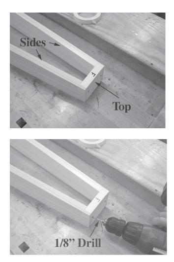
\_\_\_\_\_4. When the pilot holes are all drilled, remove the tape and put glue in the joints before installing 1-5/8" screws to draw the parts together permanently. Glue and screw both the **TOP** (2 screws) and **BASE** (4 screws) pieces to the sides. The screws should pull the parts together fully so that some glue squeezes out of the joints.
