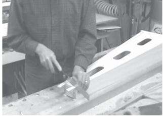
\_\_\_\_\_21. Now you need to fit the **TOP CAP** to the top of the harp body. To prepare the box for a good fit, you will need to sand the top nice and flat. The goal is to get the **FRONT**, **BACK**, and all the **TRIM** pieces flush with the two **SIDES**. It is not necessary to sand all the way down to meet the **TOP** piece -- it's easier to allow that to be slightly recessed.
