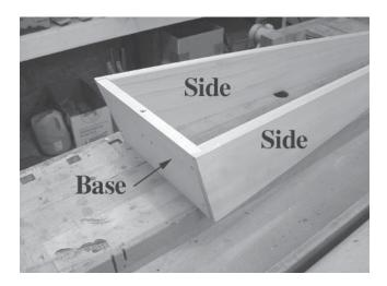
3. When the parts are properly aligned and held firmly with tape, use the smaller (1/8") drill bit provided in the kit to drill pilot holes into the **SIDES** for the screws. Aim your drill through the pre-drilled holes in the **TOP** and **BASE**. The holes you drill will guide the screws and make it much easier to screw them in without splitting the wood.
